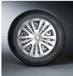
GL 15 inch steel wheels with full wheel cap
